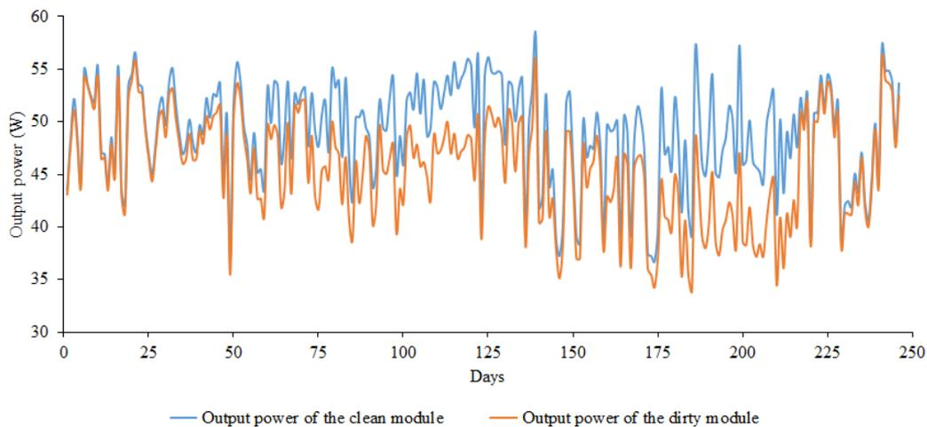
**Figure 4.** Output power of the two modules during the experimental period
