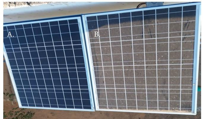
**Figure 3.** Photovoltaic modules - module cleaned weekly (A) and not cleaned, with accumulated dirt on the 177<sup>th</sup> day of the experiment (B)
