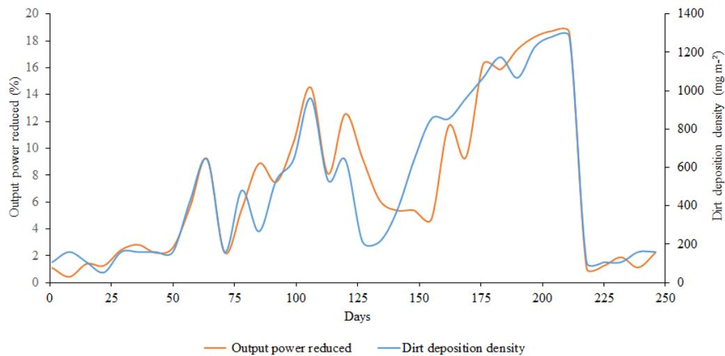
**Figure 5.** Reduced output power and dirt deposition density during the experimental period
