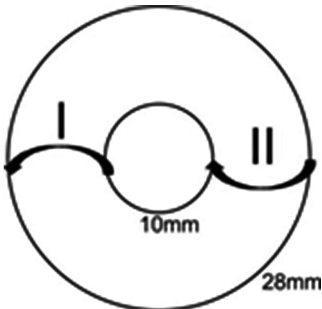
Fig. 2 - Illustration of the cycle relaxation (I) / activation (II) to which the pulsatile stent is subjected
