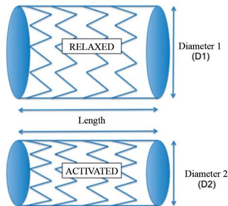
$$\text{Endoprosthesis relaxed volume: } V_1 = \frac{D_1^2}{4} \pi C$$
