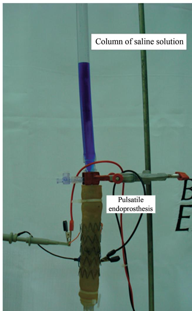
Fig. 3 - Mounting the pulsatile endoprosthesis with 5 stents connected in series in system of pulse generator, oscilloscope and current source
