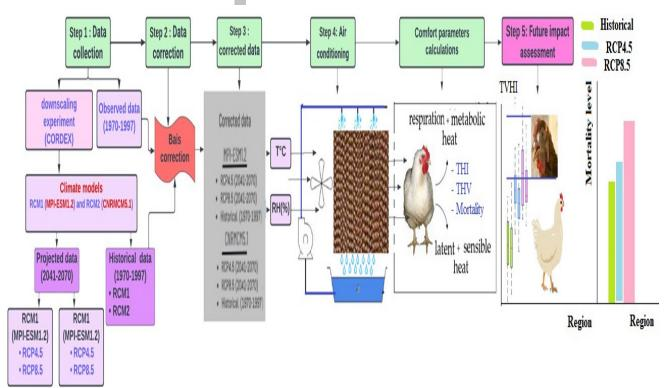
Figure 2 – Conceptual flowchart illustrating the methodology adopted for the evaluation of historical and future comfort conditions, as well mortality levels of broiler chickens when adopting a DCP system.
