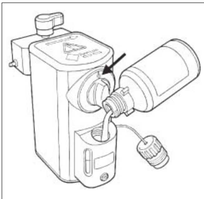
Figure 3 – Non-Specific Traditional System Type Funnel-Fill. The illustration of the Delta Vaporizer, Pour fill type, was reproduced with permission of Penlon Ltd, Abingdon, UK.
