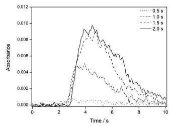
**Figure 1.** Overlaid transient signals for 1.0 mg  $L^1$  Cu at different injection times. Microemulsion composition: 1.7g of enriched sample B-01, 1100  $\mu$ L aqueous phase (1.4 mol  $L^1$  HNO<sub>3</sub>) and n-propanol (up to 10 mL). Instrumental parameters at Table 1
