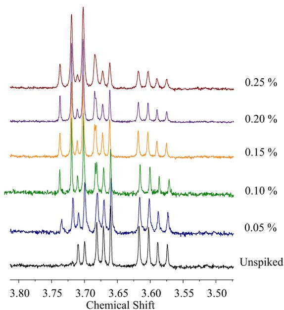
**Figure 2.**  $^1\text{H-NMR}$  spectra detail (Varian Oxford 400 MHz,  $\text{CDCl}_3$ ) of EtOH unspiked and spiked ethyl biodiesel (0.05 to 0.25%)
