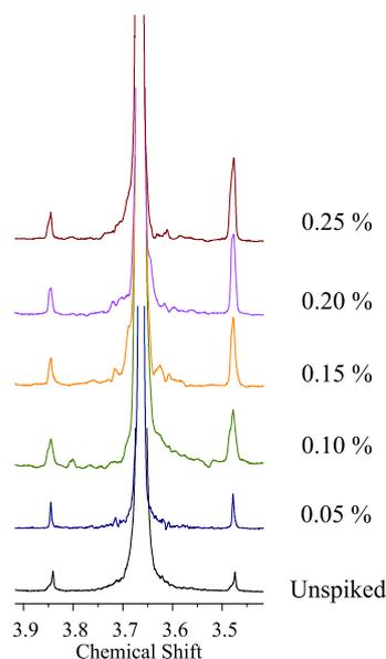
**Figure 1.**  $^1\text{H-NMR}$  spectra detail (Varian Oxford 400 MHz,  $\text{CDCl}_3$ ) of MeOH unspiked and spiked methyl biodiesel (0.05 to 0.25%)
