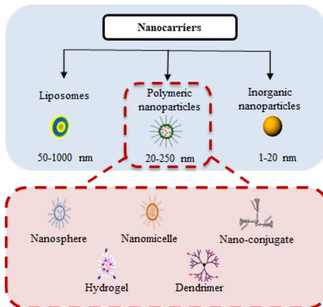
Figure 3. Types of nanocarriers<sup>7,15</sup>
