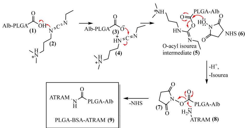
Figure 5. Coupling mechanism of ATRAM to PLGA-BSA via carbodiimide reaction<sup>57,58</sup>
