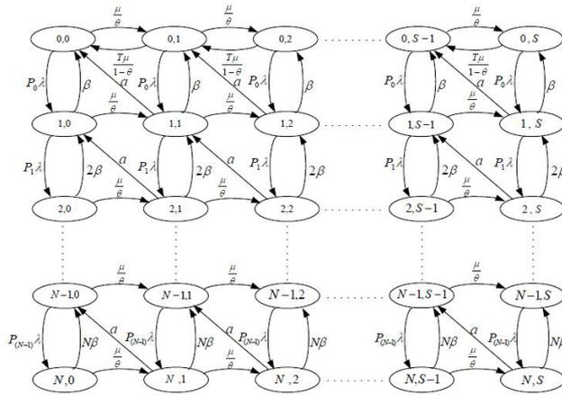
Figure 5. Second scenario state transition rates diagram.
