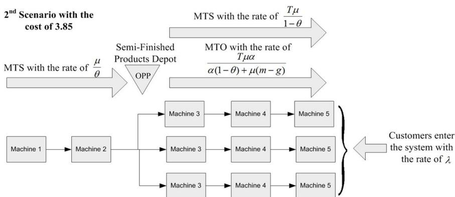
Figure 6. Production line related to second scenario in the numerical example (MTS = Make to Stock; MTO = Make to Order).
