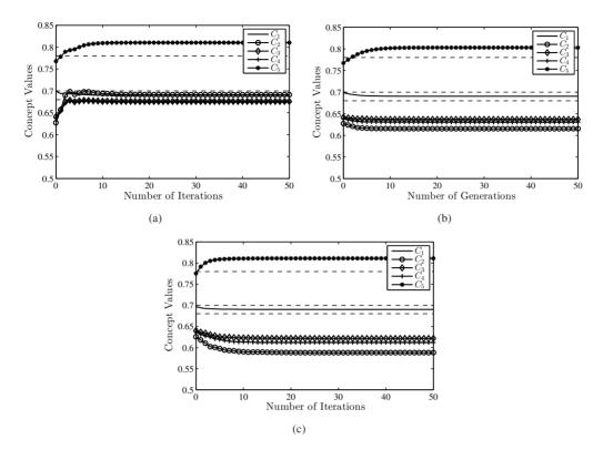
**Figure 10** – Mean convergence for Scenario 4 in PROC1 considering (a) PSO, (b) GA and (c) ACO with  $\mathcal{P} = M = 10$ .
