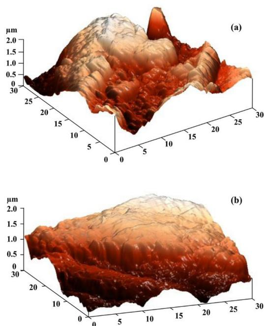
**Figure 3.** Atomic force microscopy (AFM) images of (a) AVF and (b) PANI-COATED:AVF.
