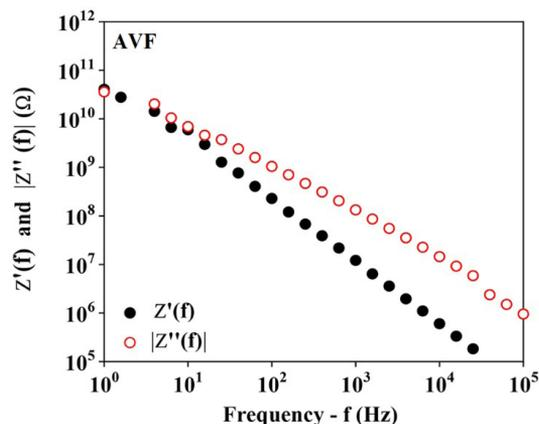
Figure 6. Real,  $Z'(f)$ , and imaginary,  $Z''(f)$ , components of the complex impedance versus frequency ( $f$ ) of AVF.
