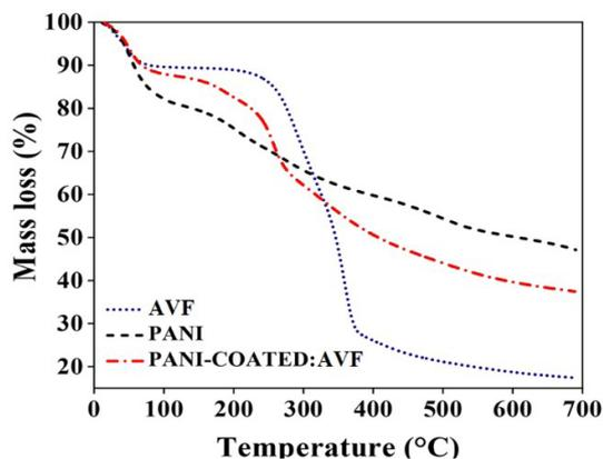
Figure 5. Thermogravimetric analysis (TGA) curves of samples AVF, PANI, and PANI-COATED:AVF.
