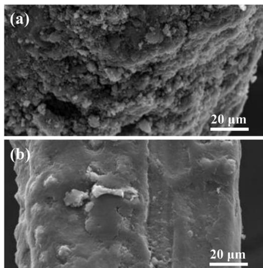
**Figure 2.** Scanning electron microscopy (SEM) images of (a) AVF and (b) PANI-COATED:AVF.
