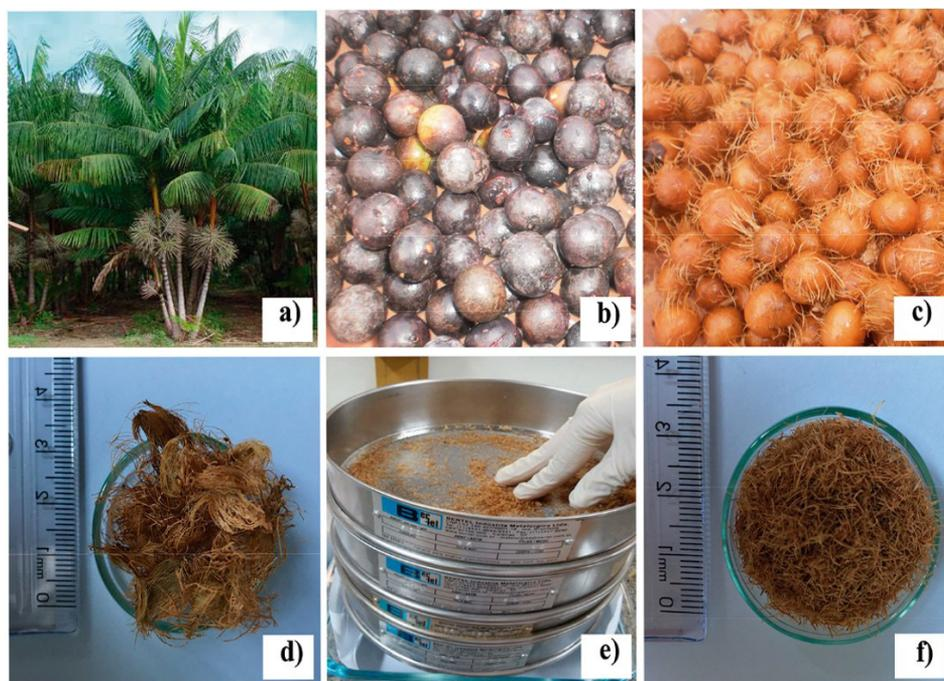
**Figure 1.** Preparation of acai vegetable fibers (AVF). (a) Amazonian palm; (b) açai fruit; (c) açai waste after depulping; (d) AVF; (e) AVF sieving; (f) AVF with a length of  $3.0 \pm 1.0$  mm.
