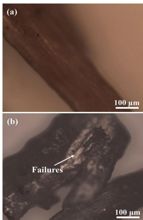
**Figure 4.** Optical microscopy (OM) images of (a) AVF and (b) PANI-COATED:AVF.
