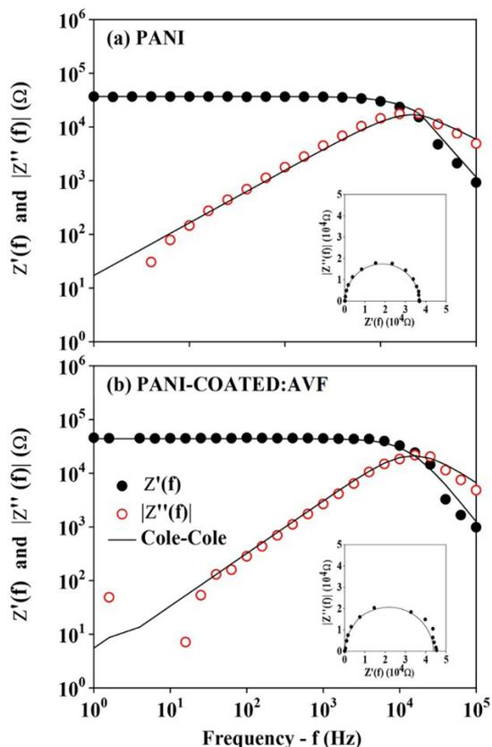
Figure 7.  $Z'$  and  $Z''$  vs.  $f$  of (a) PANI and (b) PANI-COATED:AVF. The inset image shows an Argand diagram of the  $Z'(f)$  vs.  $Z''(f)$  of (a) PANI and (b) PANI-COATED:AVF. The full lines represent the experimental fittings obtained from Equation 1.
