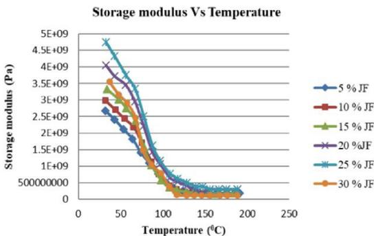
Figure 10. Storage Modulus of Jute fibre reinforced polyester/clay nanocomposites at 10Hz frequency.
