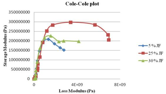
Figure 16. Cole-Cole plot of the Jute fibre reinforced polyester/ clay nanocomposites at 10Hz frequency.
