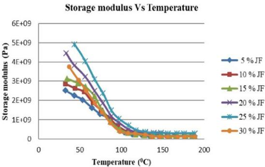
Figure 9. Storage Modulus of Jute fibre reinforced polyester/clay nanocomposites at 5Hz frequency.
