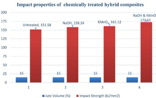
**Figure 5.** Comparison of the impact properties of chemically treated jute fibre reinforced polymer composites with 5wt% montmorillonite clay as filler.
