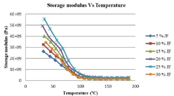
**Figure 6.** Storage Modulus of Jute fibre reinforced polyester/clay nanocomposites at 0.5Hz frequency.
