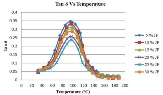
Figure 12. Effect of Tanδ at 1Hz frequency on Jute fibre reinforced polyester/clay nanocomposites.
