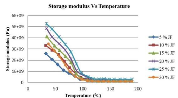
**Figure 7.** Storage Modulus of Jute fibre reinforced polyester/clay nanocomposites at 1Hz frequency.
