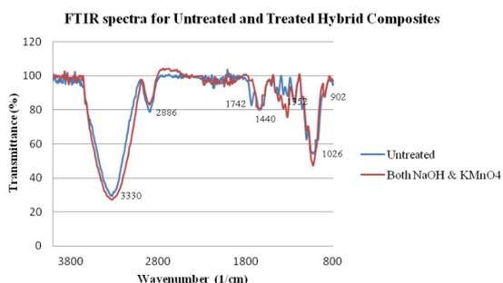
**Figure 2.** FTIR spectra curve for untreated and chemically treated NaOH and  $\text{KMnO}_4$  fibre.
