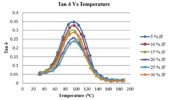
Figure 11. Effect of Tanδ at 0.5Hz frequency on Jute fibre reinforced polyester/clay nanocomposites.
