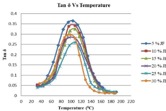
Figure 15. Effect of Tanδ at 10Hz frequency on Jute fibre reinforced polyester/clay nanocomposites.
