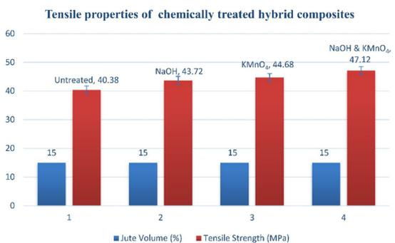
**Figure 3.** Comparison of the tensile properties of chemically treated jute fibre reinforced polymer composites with 5wt% montmorillonite clay as filler.
