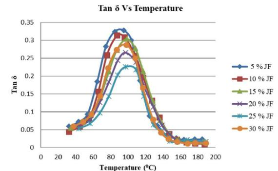
Figure 13. Effect of Tanδ at 2Hz frequency on Jute fibre reinforced polyester/clay nanocomposites.
