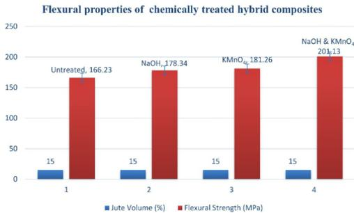
**Figure 4.** Comparison of the flexural properties of chemically treated jute fibre reinforced polymer composites with 5wt% montmorillonite clay as filler.
