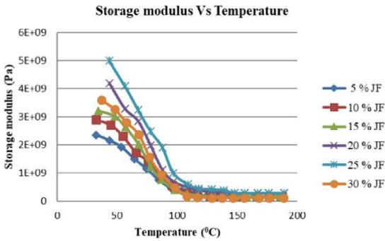
Figure 8. Storage Modulus of Jute fibre reinforced polyester/clay nanocomposites at 2Hz frequency.
