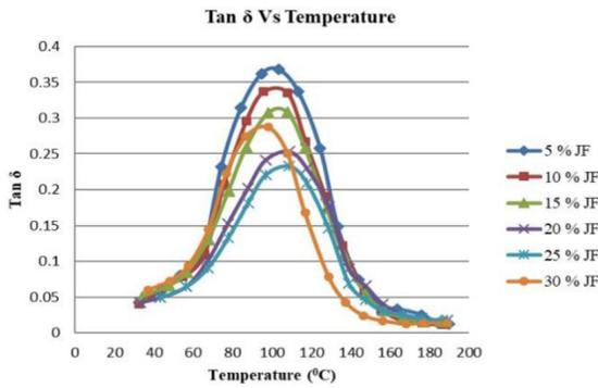
Figure 14. Effect of Tanδ at 5Hz frequency on Jute fibre reinforced polyester/clay nanocomposites.
