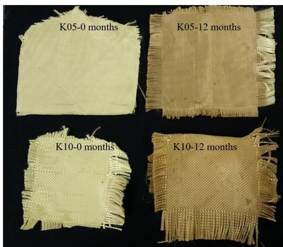
**Figure 5.** Color changes of the samples before and after natural ageing.
