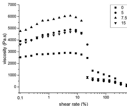
Figure 8. Viscosity as a function of shear rate for PA/SEBS non-compatibilized and compatibilized blends.
