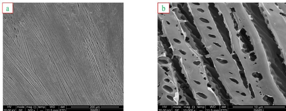
**Figure 6.** SEM images of AM/SSS/THDAB: 1000×, scale bar 200 μm (a) 10000×, scale bar 50 μm (b).
