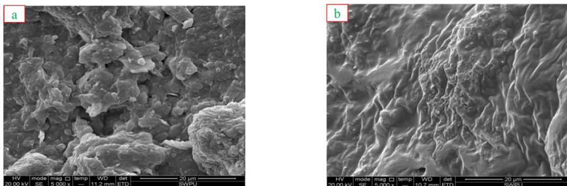
Figure 8. SEM observations of Na-MMT composites (×5000): (a) basic muds cake; (b) treated with 2 wt% AM/SSS/THDAB.
