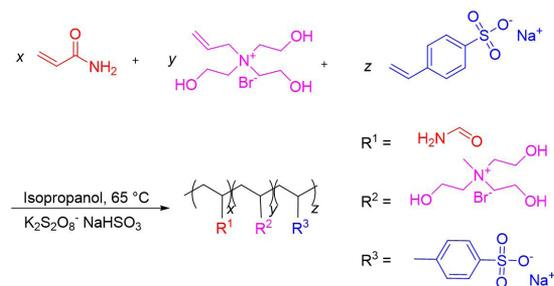
Figure 2. Synthesis route of AM/SSS/THDAB.
