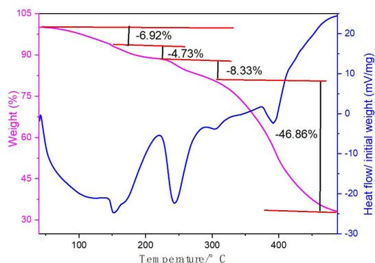
Figure 5. TGA-DSC measurement of AM/SSS/THDAB.
