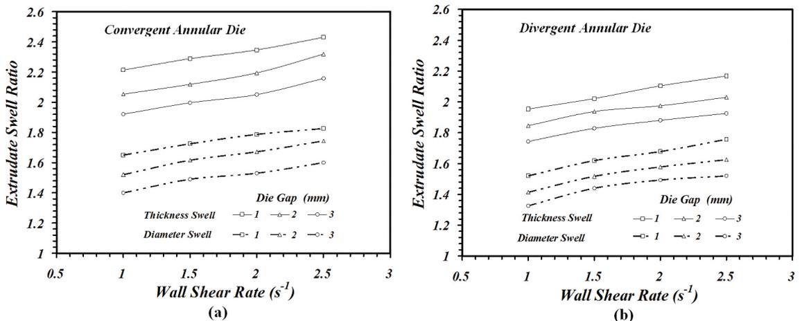
**Figure 7.** Diameter swell and thickness swell of NR compound flowed from the convergent annular die (a) and the divergent annular die (b) with different die gap [1 mm, 2 mm, 3 mm].
