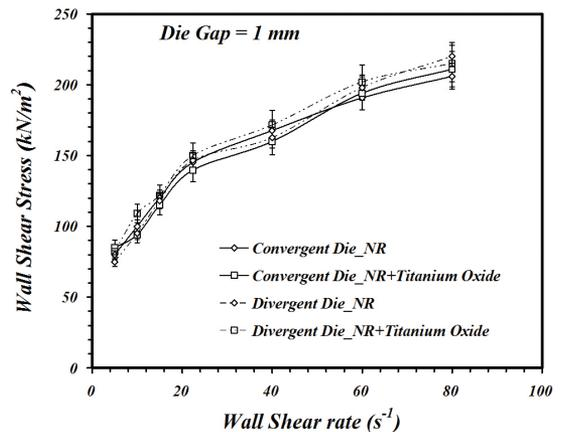
**Figure 4.** Flow curves of NR compound with and without addition of Titanium Oxide pigment from convergent and divergent annular die with the die gap of 1 mm.
