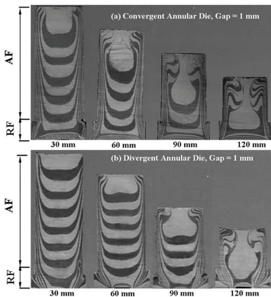
**Figure 5.** Flow patterns of NR compound in the barrels of convergent annular die system (a) and divergent annular die system (b) with different piston displacements [30 mm, 60 mm, 90 mm, 120 mm] and shear rate of  $1.5\text{ s}^{-1}$ .
