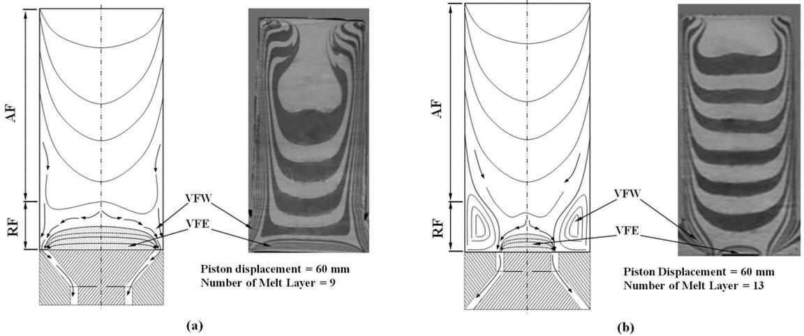
**Figure 6.** A schematic flow drawing for NR compound in the barrels of convergent annular die system (a) and divergent annular die system (b) with piston displacements of 60 mm.
