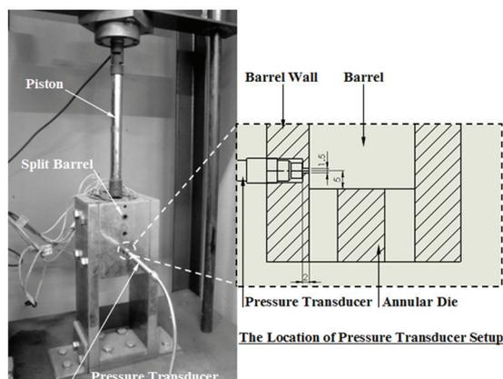
**Figure 1.** The split barrel constant shear rate capillary rheometer.
