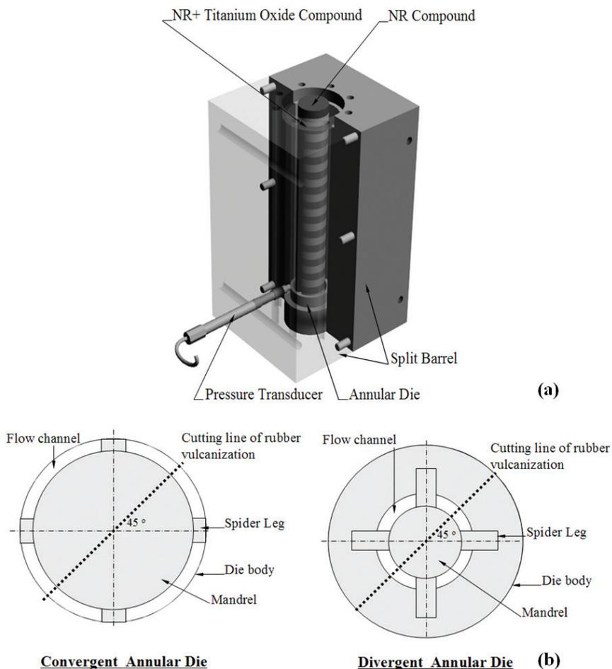
Figure 3. An experimental arrangement for the Colored Layer Technique (a) the tops of divergent annular die and convergent annular die show the cutting line of rubber vulcanization rod (b).
