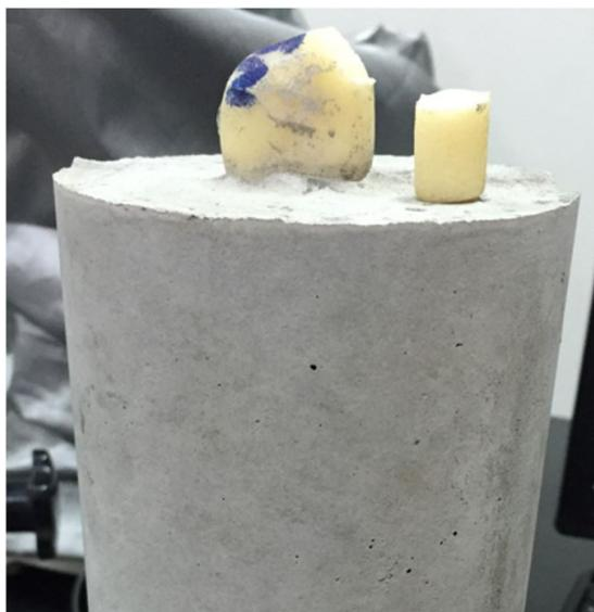
Figure 9. Fracture of the neck of the femoral stem without a center.
