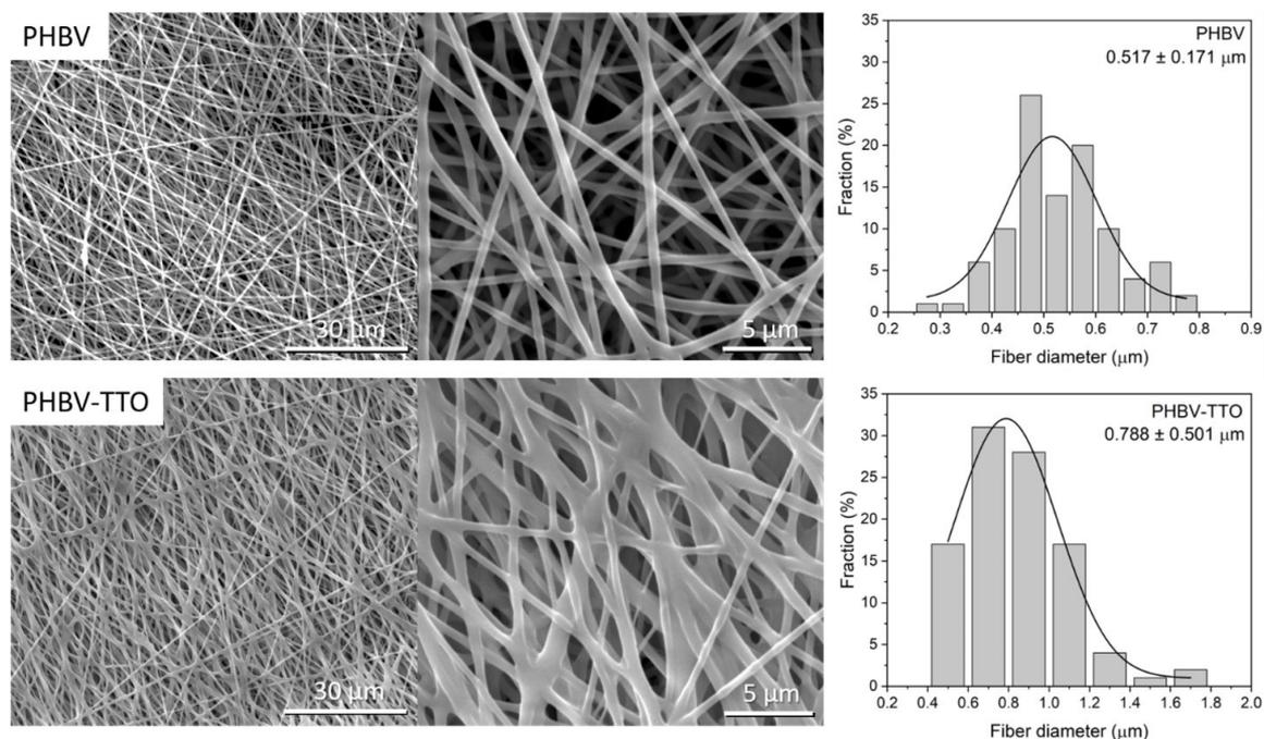
**Figure 1.** SEM images and fiber diameter distribution of PHBV and PHBV-TTO nanofibers.
