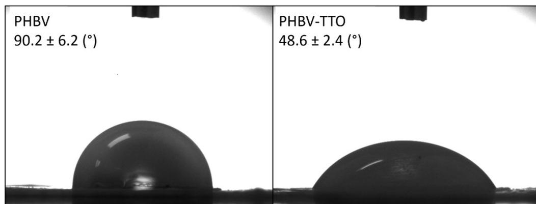
Figure 2. Water contact angle of the PHBV and PHBV-TTO nanofibers.
