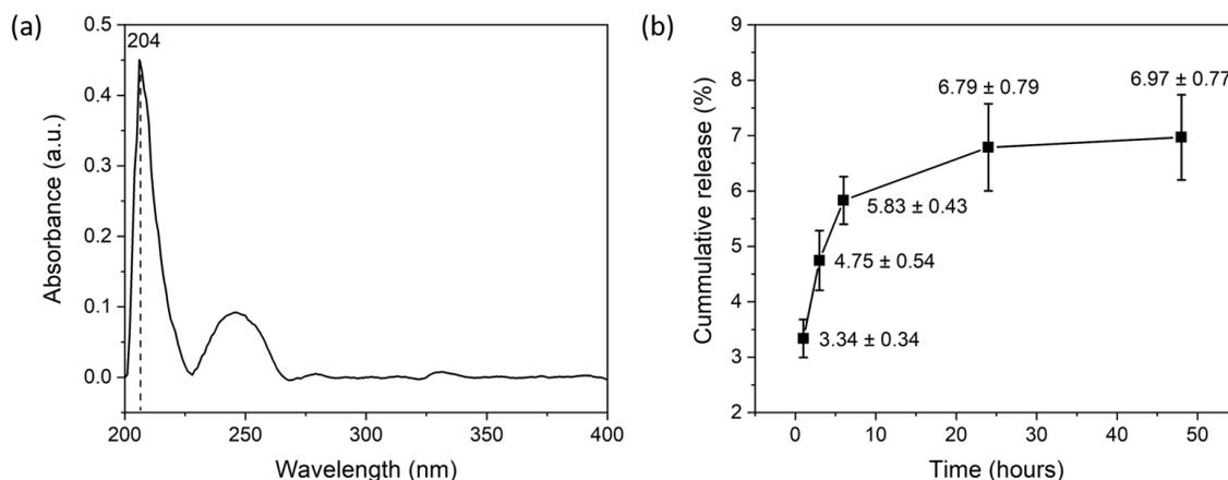
**Figure 4.** (a) Representative UV-vis spectra from the aliquots and (b) cumulative release of TTO from PHBV-TTO nanofibers (1, 3, 6, 24, and 48 hours).
