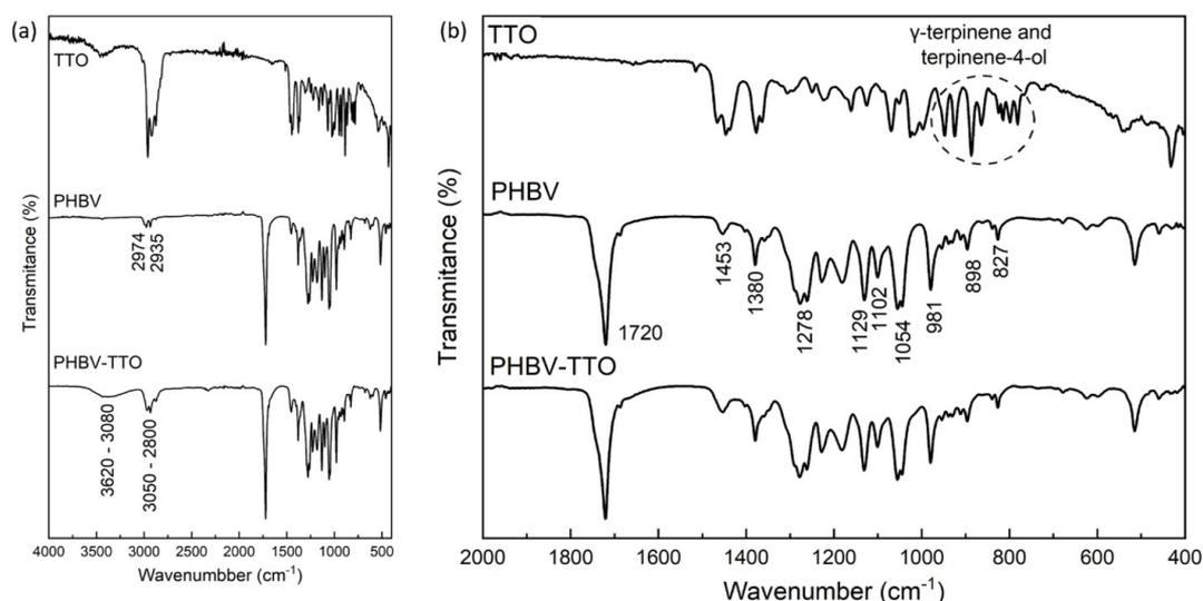
Figure 3. FTIR spectra of pure TTO, PHBV and PHBV-TTO. (a) 4000-400  $\text{cm}^{-1}$  and (b) 2000-400  $\text{cm}^{-1}$ .
