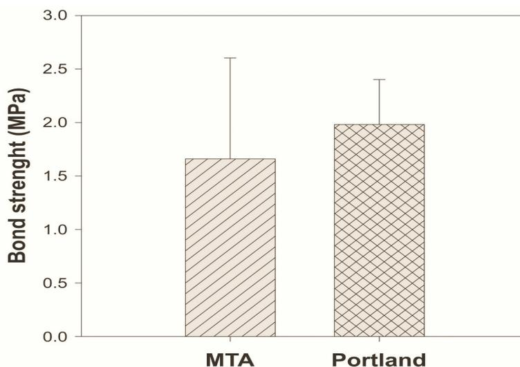
**Figure 2. Push-out strength values (means) for each cement.**
