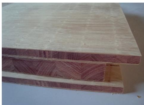
Figure 3. Experimental panels of eucalyptus laths coated with bamboo veneer (Source: Ostapiv 2011).
