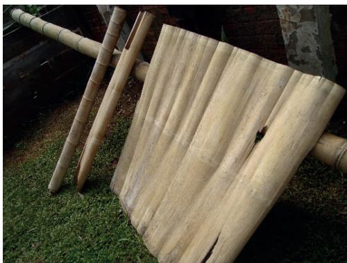
Figure 1. *Dendrocalamus asper* veneers obtained by centerless grinding (Source: Ostapiv 2011).
