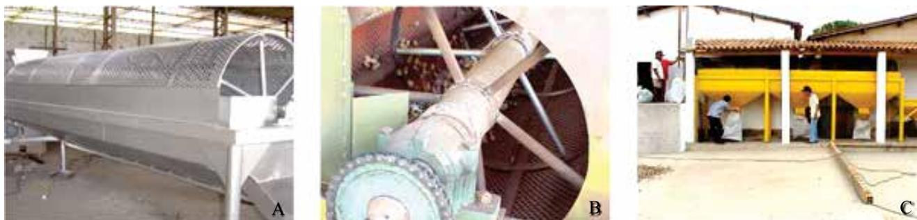
**Figure 1.** Sorting cashew (*Anacardium occidentale*) nuts by size: A, general view of the sorter; B, sorter with nuts during the sorting process; C, nuts being placed in the sorter and removed by size. Photo by Cláudio de Norões Rocha.
