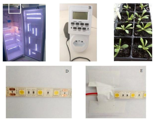
**Figure 9.** Installation of LED strips spaced inside the refrigerator. Highlighted in the image is the external / internal access to the installation of the LED strips (A). Digital timer used to turn the LED lights on and off inside the refrigerator (B). Statice seedlings with approximately five true leaves, when they were placed into the BOD prototype (C). LED strips: (D) a segment of the LED strip; (E) soldering point with adhesive tape finish.
