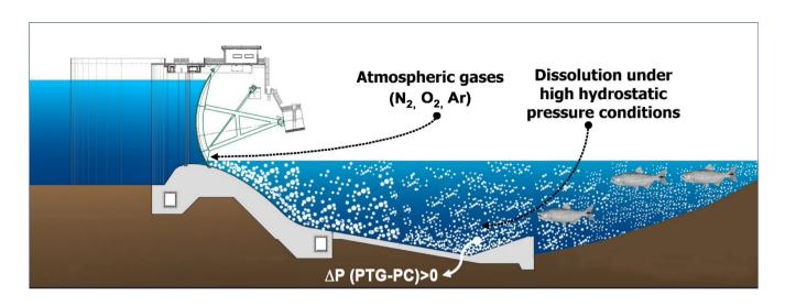
**FIGURE 1** | Processes involved in gas supersaturation at downstream a spillway. PTG = Total gas pressure, PC = Compensation Pressure (barometric + hydrostatic) – (modified from Abernethy *et al.*, 2001).
