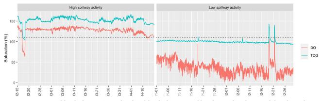
**FIGURE 3** | Saturations of dissolved oxygen (DO, red) and total dissolved gases (TDG, blue), for periods with intense (left) and sporadic (right) dam spillway activities. The black dotted line indicates the threshold of 110% TDG saturation.
