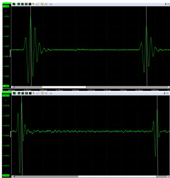
**Figure 5.** Echo signal of a longitudinal wave (top) and a shear wave (bottom).
