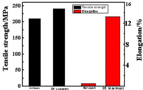
**Figure 4.** Variations in tensile strength, and elongation of as-cast A390-0.3wt.%Nd and extrusion and heat treatment samples
