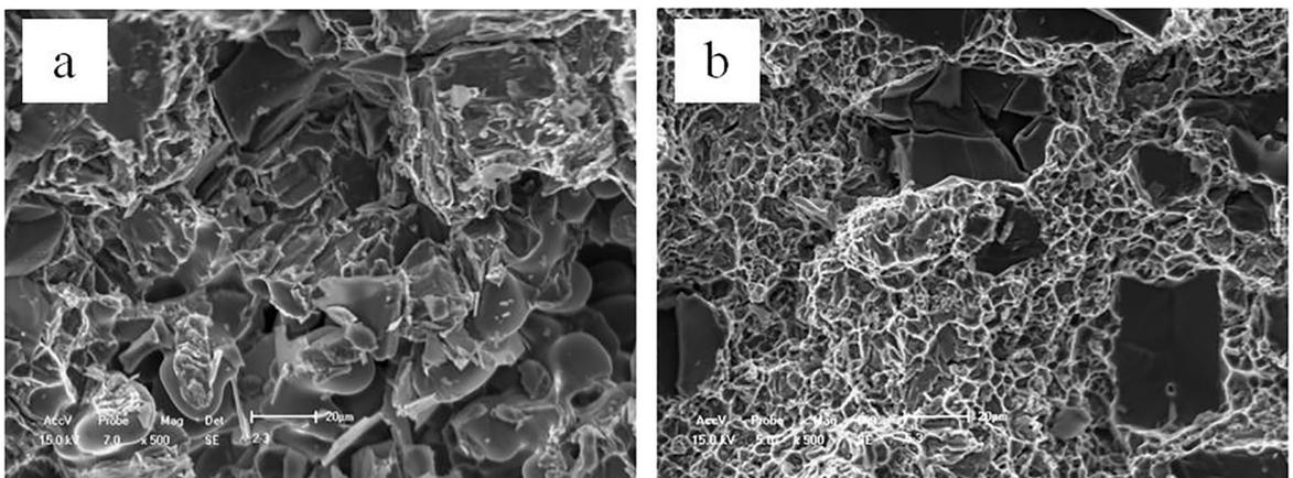
**Figure 5.** The SEM images of fracture surfaces of (a) as-cast A390-0.3Nd alloy sample; and (b) extruded and heat treated sample of A390-0.3wt%Nd alloy
