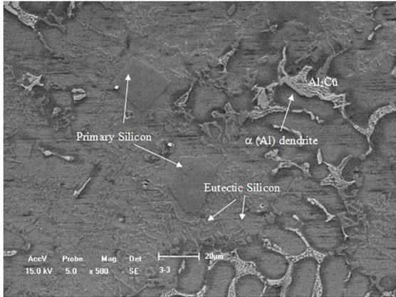
Figure 1. SEM image of A390-0.3wt%Nd alloy
