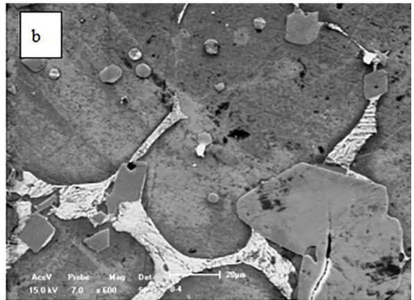
Figure 2. SEM images of A390-0.3wt%Nd alloy after heat treatment at different magnifications
