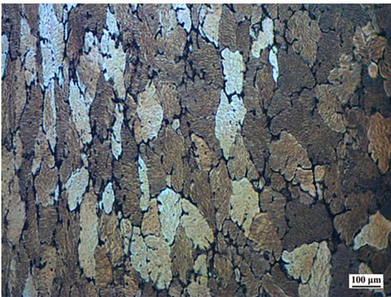
Figure 1. Original metallography for as cast AlCu4SiMg alloy.
