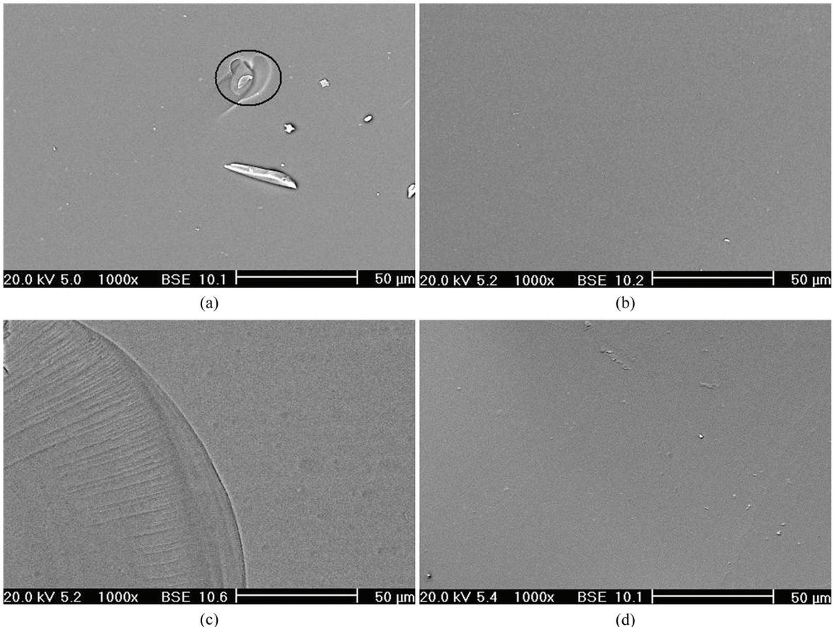
**Figure 3.** SEM images of rock wools fabricated using only granite waste (a), only steelmaking slag (b), both residues (c), and from a industrial sample (d).
