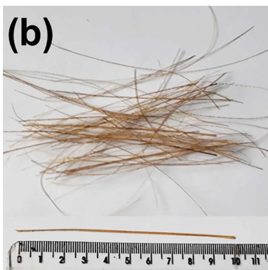
Figure 2. As received bundle of guaruman stems (a) and extracted fibers (b).
