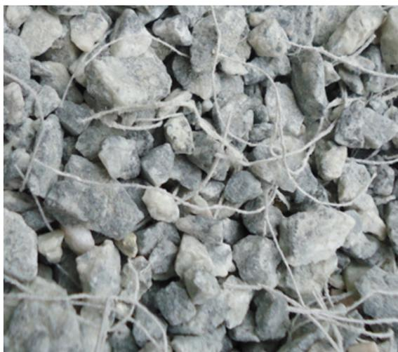
**Figure 2-** Synthetic macrofibres interlaced to the aggregates after the mixing process
