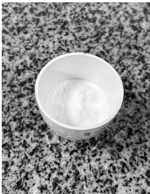
Figure 1. SBA-15, obtained after calcination.
