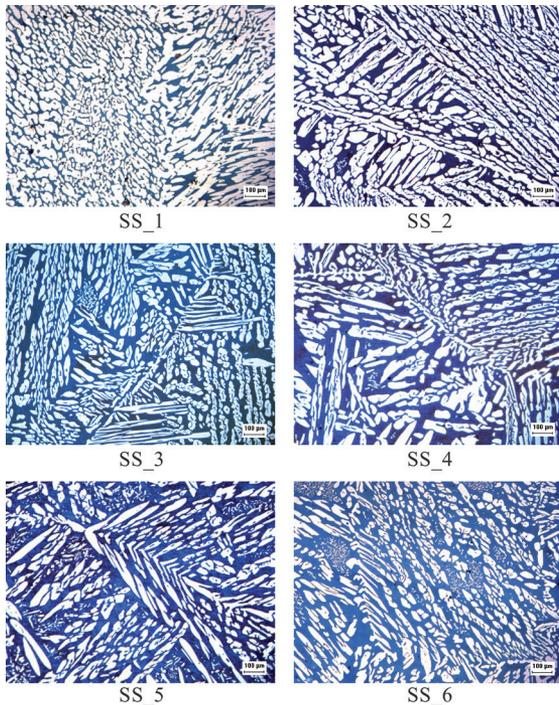
**Figure 1:** Microstructures of austenitic-ferritic steels after Beraha's etch. Microscopy magnifications: 100X.
