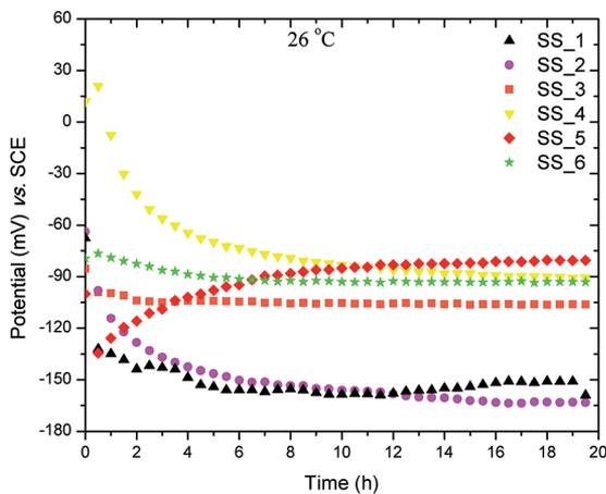
**Figure 4:** OCP (mV) versus time (hours) for all samples at room temperature in 3.5% NaCl solution.
