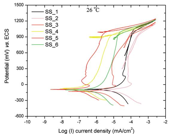
**Figure 5:** Potentiodynamic polarization curves at 26°C in 3.5% NaCl; 0.5 mV s<sup>-1</sup>.
