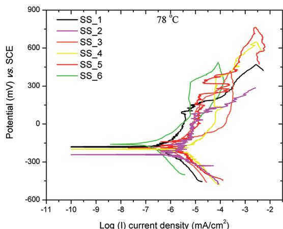
**Figure 6:** Potentiodynamic polarization curves at 78°C in 3.5% NaCl; 0.5 mV.s<sup>-1</sup>.
