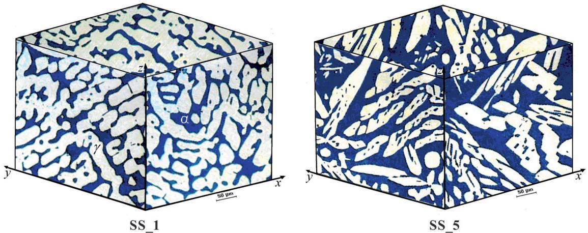
**Figure 3:** Typical microstructure of austenitic-ferrite steel in three directions for the alloy with smaller and higher ferrite %, SS\_1 and SS\_5 respectively. Microscopy magnifications: 200X.
