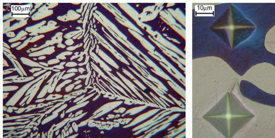
**Figure 2:** Typical microstructure of austenitic-ferritic steel (right) and Illustration of Vickers microhardness indentation in the ferrite (dark phase) (left), (Microscopy magnifications: 100X and 500X, respectively).
