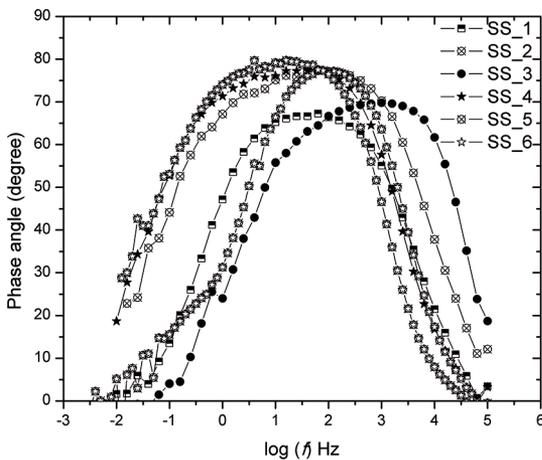
**Figure 9:** Bode phase angle vs.  $\log(f)$  diagrams for all samples in 3.5 wt% NaCl solution at 25 °C.
