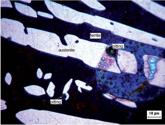
**Figure 7:** Optical micrograph of the SS\_4 steel annealed at 1100°C after potentiodynamic polarization in 3.5 wt% NaCl solution performed at 78°C, showing pitting etch advancing on the austenite phase.
