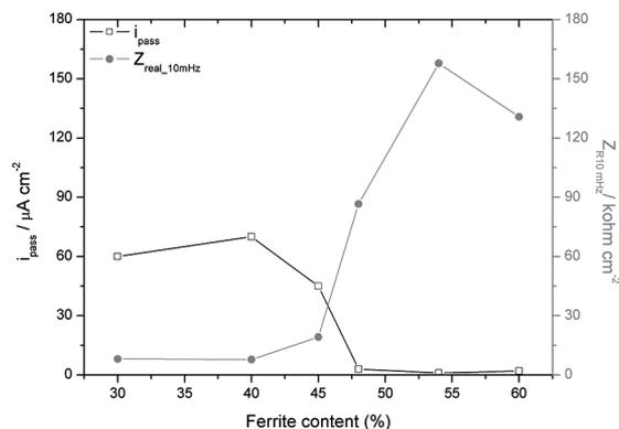
**Figure 10:** Passive current density and impedance (real part) at 10 mHz as a function of the ferrite content.
