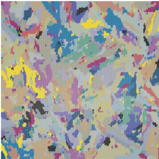
Figure 3. Polycrystalline geometric finite element model based on EBSD experimental data.
