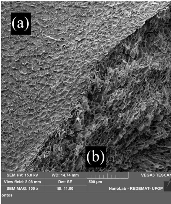
**Figure 1.** Fiber micrograph showing (a) frontal view of the epidermis of the fiber and (b) parenchymal region containing sclereids and parenchymal cells with lignified thickening bars.
