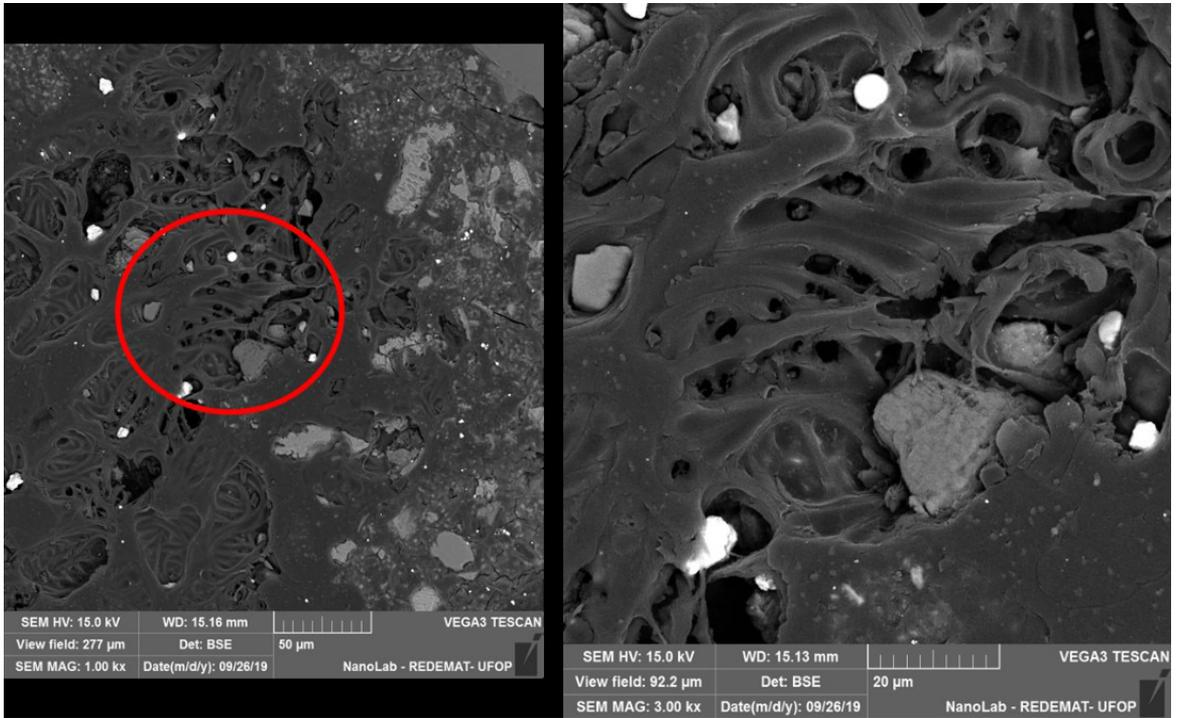
**Figure 6.** Micrograph of sample AF100-02 tested at 7 days with magnification of 1000x and 3000x.
