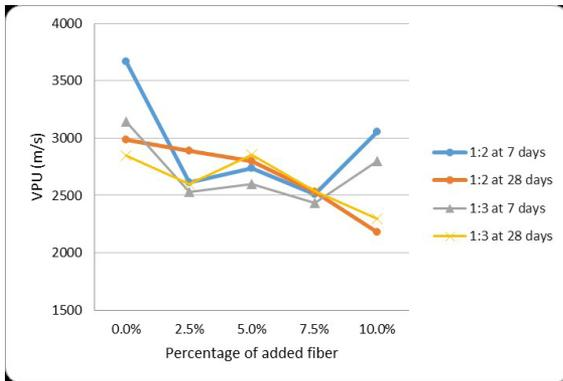
Figure 4. Average of the ultrasonic pulse propagation speed.
