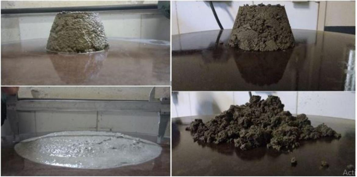
Figure 3. Comparison between the consistency of REF-02 and AF100-02 mortars.
