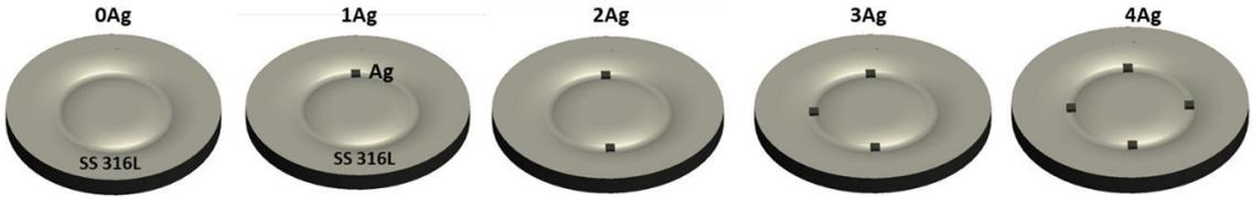
Figure 2. 316L stainless steel (SS316L) target doped with inserts of Ag (0, 1, 2, 3, and 4 inserts).
