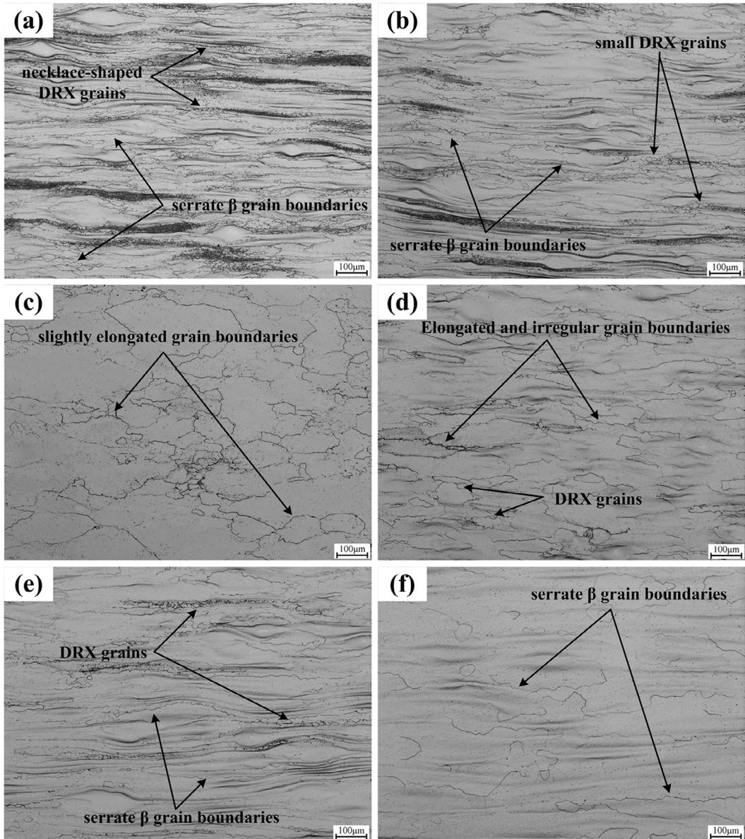
**Figure 6.** Optical microstructures of deformed PM Ti-5553 alloy subjected to various temperatures and deformation strain at  $1 \text{ s}^{-1}$  near the  $\beta$  transus and in  $\beta$  region: (a)  $950 \text{ }^\circ\text{C}$ , 70%; (b)  $1000 \text{ }^\circ\text{C}$ , 70%; (c)  $1050 \text{ }^\circ\text{C}$ , 30%; (d)  $1050 \text{ }^\circ\text{C}$ , 50%; (e)  $1050 \text{ }^\circ\text{C}$ , 70%; and (f)  $1150 \text{ }^\circ\text{C}$ , 70%.
