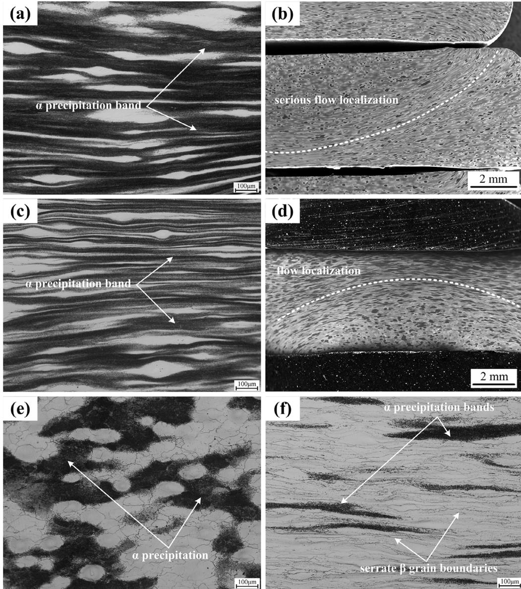
**Figure 4.** Optical microstructures and SEM characteristics of deformed PM Ti-5553 alloy subjected to various temperatures and deformation strain at  $1 \text{ s}^{-1}$  in  $(\alpha+\beta)$  region: (a) OM, 700 °C, 70%; (b) SEM, 700 °C, 70%; (c) OM, 800 °C, 70%; (d) SEM, 800 °C, 70%; (e) OM, 900 °C, 30%; and (f) OM, 900 °C, 70%
