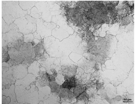
**Figure 1.** Optical image showing the origin microstructure of as-consolidated PM Ti-5553 alloy
