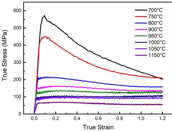
**Figure 2.** True stress-stain curves of as-consolidated PM Ti-5553 alloy at 1 s<sup>-1</sup> and various temperatures
