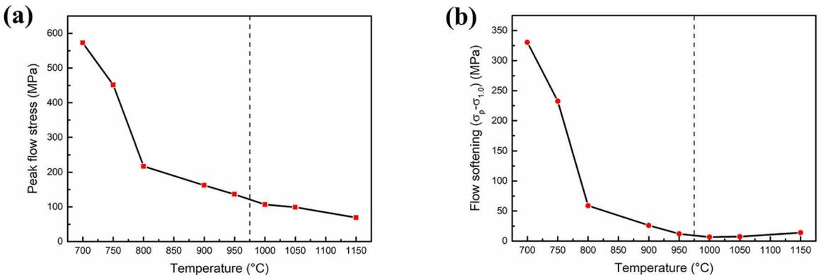
**Figure 3.** The changing of peak flow stress and flow softening values of as-consolidated PM Ti-5553 alloy with temperature of during hot deformation: (a) peak flow stress; and (b) flow softening ( $\sigma_p - \sigma_{1.0}$ ) value
