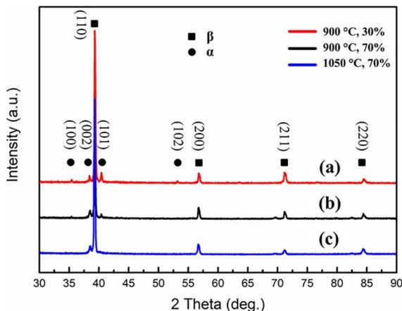
**Figure 5.** XRD patterns of deformed PM Ti-5553 alloy subjected to various temperatures and deformation degrees at  $1 \text{ s}^{-1}$ : (a) 900 °C, 30%; (b) 900 °C, 70%; and (c) 1050 °C, 70%
