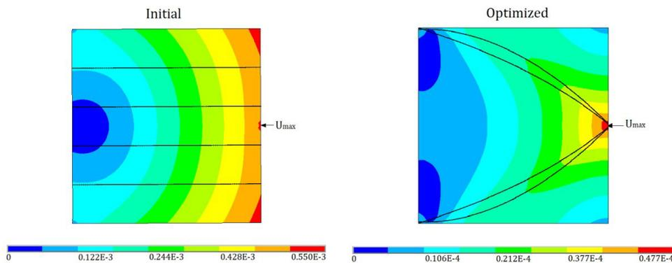
**Figure 7** Initial and Final structures initial fiber inclination of 0°
