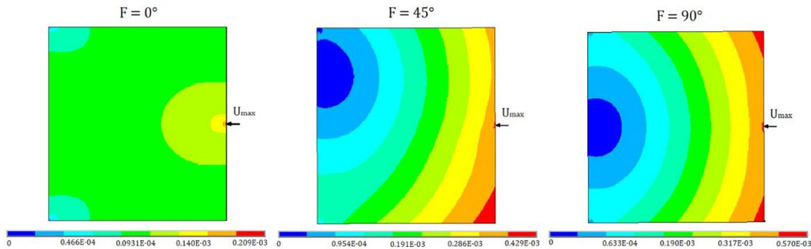
Figure 4 Displacement fields in structures without reinforcements
