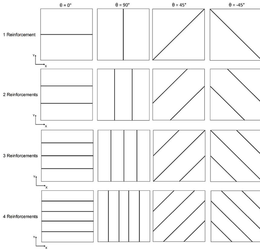
**Figure 1** Initial angle and position of the reinforcements in the cases studied
