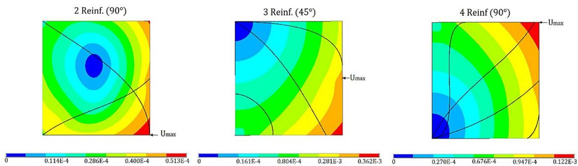
Figure 6 - Distribution of displacements in reinforcements with different number of reinforcements and initial inclination
