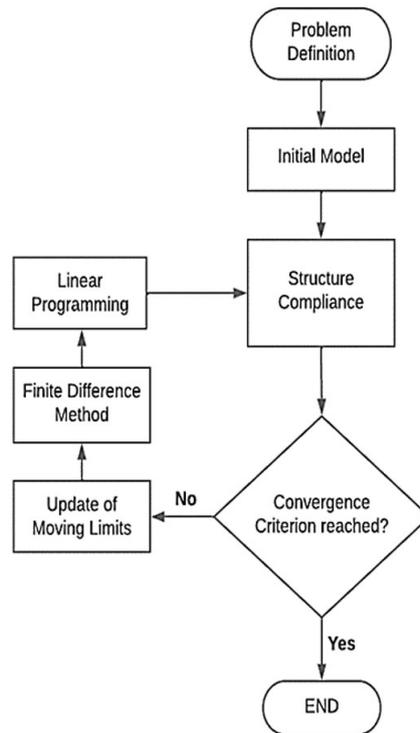
**Figure 3** Structure optimization flowchart
