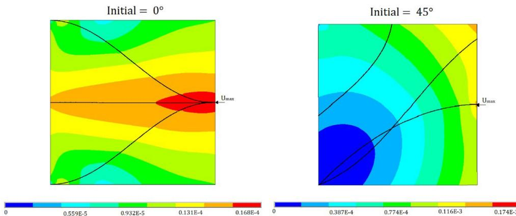
Figure 5 Distribution of displacements in structures with three reinforcement and different initial fibers slope
