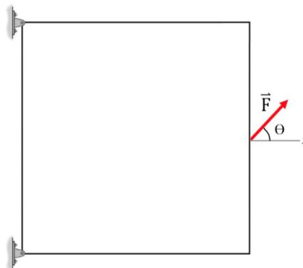
**Figure 2** Support conditions and loading
