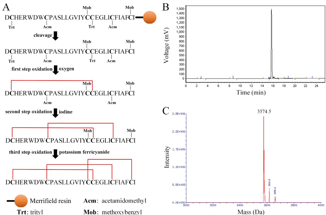
**Figure 2.** Synthesis and confirmation of Tx6.7. **(A)** Schematic representation of the disulfide bond synthesis of Tx6.7. **(B)** Purification of Tx6.7 by reverse-phase HPLC. **(C)** Mass spectra of Tx6.7.
