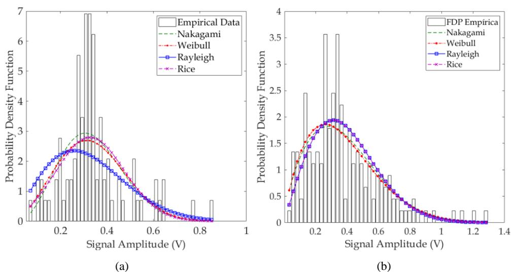
Fig. 6. Small scale fading statistics (a) LOS Situation and, (b) NLOS Situation
