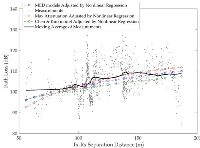
Fig. 8. Result of the models fitted by OLS nonlinear regression.
