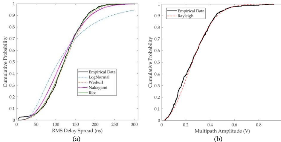
Fig. 11. Cumulative distribution function of (a) the RMS delay spread and (b) the amplitude of multipath.
