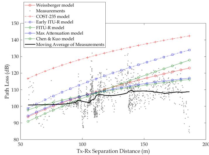
Fig. 7. Models fitted to the measurements.
