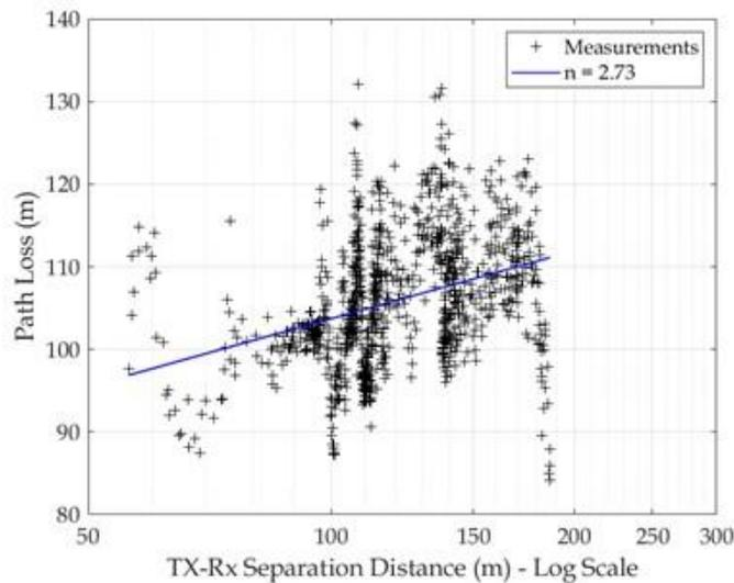
Fig. 5. Measurements and path loss adjusted to the data.
