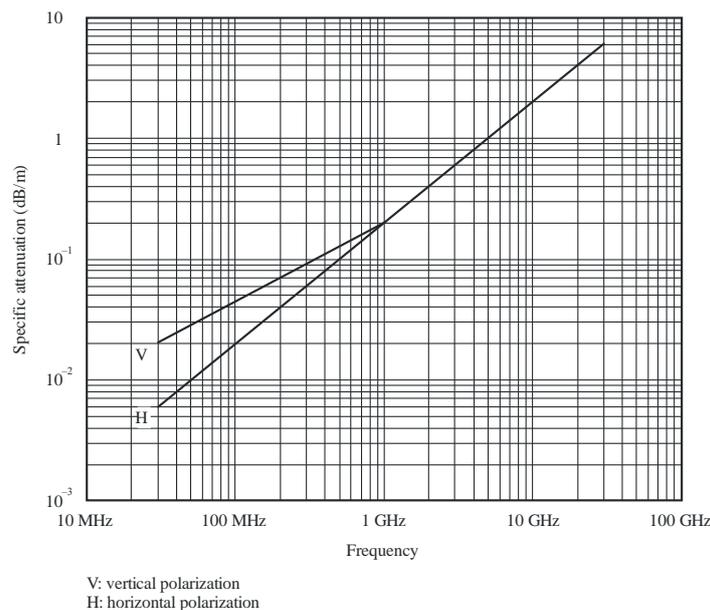
Fig. 2. Specific attenuation due to vegetation, in dB/m, as a function of frequency [15].
