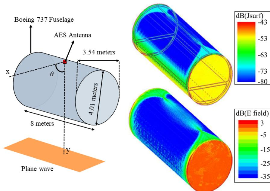
Fig. 1. Aircraft fuselage electromagnetic numerical current density and electric field.
