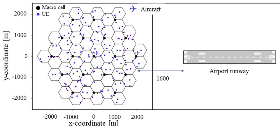
Fig. 3. Simulation scenario between IMT-2020 Base Stations and AES.
