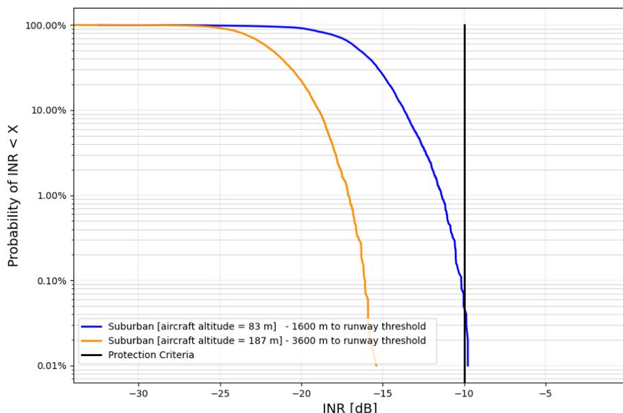
Fig. 5. CDF of interference over noise ratio (INR) received from IMT-2020 (10000 snapshots).
