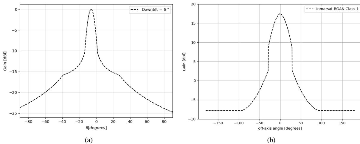
Fig. 4. Antenna models used in the simulation. (a) IMT Suburban Base Station (normalized), (b) Inmarsat-BGAN Class 1.
