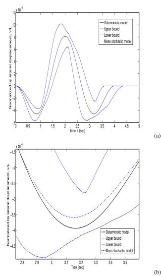
Figure 8. (a) Tip displacement history for a composite beam that rotates following Eq. (39), for  $\delta_{V_i} = 0.05$  in all variables, (b) a detail.
