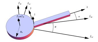
Figure 1. Reference frames of the rotating beam.
