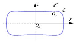
Figure 2. Reference frames of the cross-section.
