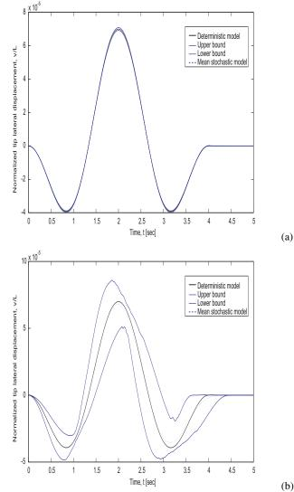
Figure 9. Tip displacement history of a composite beam that rotates following Eq. (39) for  $\delta_{V_i} = 0.05$  (a) only in random variable  $V_3$ , (b) in random variables  $V_5$  and  $V_6$ .
