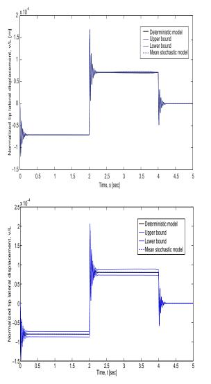
Figure 6. Tip displacement history for a composite beam that rotates following Eq. (38), for  $\delta_{V_i} = 0.05$  (a) only in random variable  $V_3$ , (b) only in random variable  $V_4$ .
