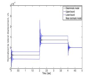
Figure 5. Tip displacement history for a composite beam that rotates according to Eq. (38), for  $\delta_{V_i} = 0.1$  in all variables.
