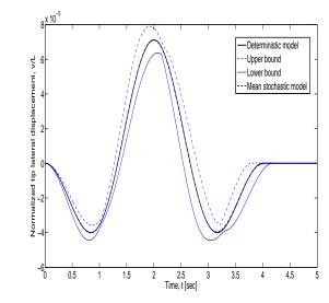
Figure 7. Tip displacement history for a composite beam that rotates following Eq. (39), for  $\delta_{V_i} = 0.02$  in all variables.
