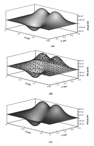
Figure 5. Static displacement distribution obtained by using the closed form solution (a), the finite element technique (b), and software ANSYS<sup>®</sup> (c).
