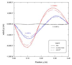
Figure 12. Comparison of the dynamic displacement distribution (section  $x = L_x/2$ ) at time instants: 0.005 s, 0.01 s, and 0.02 s.
