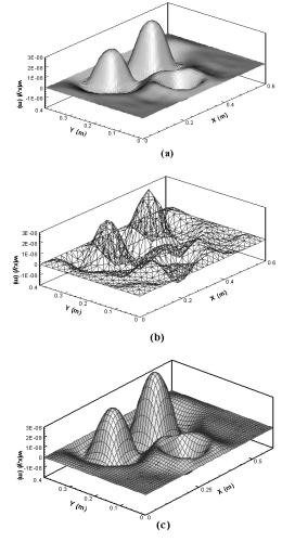
Figure 8. Dynamic displacement distribution (at 0.005 s) obtained by using closed form solution (a), the present finite element technique (b), and software  $ANSYS^{\Phi}$  (c).
