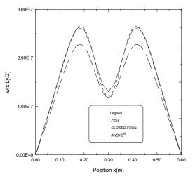
Figure 6. Comparison of the static displacement distribution (section  $y = L_y/2$ ) for the numerical techniques presented.
