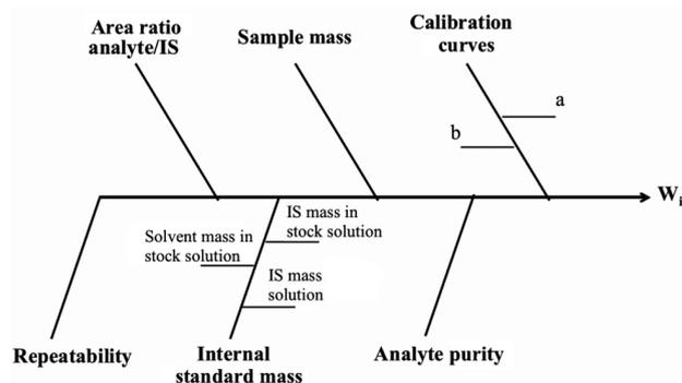
**Figure 3.** Cause-and-effect diagram of characterization uncertainty sources.
