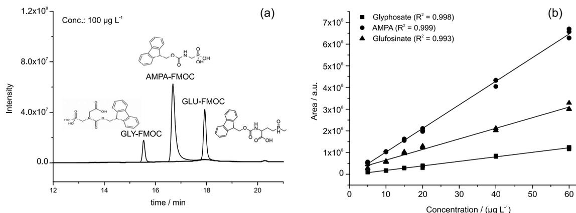
**Figure 2.** Chromatogram (a) and analytical curve (b) of the derivatives GLY-FMOC, AMPA-FMOC, and GLU-FMOC.
