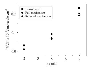
Figure 5. Simulated and experimental data for the peroxyacetyl nitrate (PAN) concentrations as a function of reaction time.
