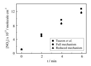
Figure 7. Simulated and experimental data for the NO<sub>2</sub> concentrations as a function of reaction time.
