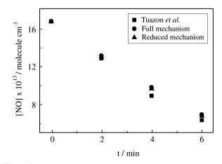
Figure 6. Simulated and experimental data for the NO concentrations as a function of reaction time.
