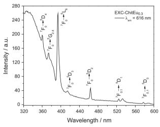
**Figure 6.** Excitation spectrum of the sample  $ChiEu_{0.3}$  measured by monitoring the emission at 616 nm. The characteristic transitions of  $Eu^{III}$  are indicated by the respective bands.
