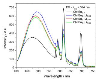
**Figure 7.** Comparison of emission spectra of samples doped with different amounts of Eu(CF<sub>3</sub>SO<sub>3</sub>)<sub>3</sub> and Li(CF<sub>3</sub>SO<sub>3</sub>)<sub>3</sub>. All the spectra were measured with excitation at 394 nm.
