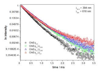
**Figure 8.** Fluorescence decay curves of  $ChiEu_{0.3}$  and  $ChiEu_{0.1}Li_n$  (n = 0.04, 0.05, 0.1 wt.%) samples determined by single exponential fittings;  $\lambda_{exc}$  = 394 nm,  $\lambda_{em}$  = 616 nm.
