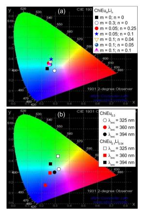
**Figure 9.** CIE chromaticity diagrams showing the (x,y) colour coordinates of emissions of ChiEu<sub>m</sub>Li<sub>n</sub> samples. In (a), the dependence on Eu<sup>3+</sup> and Li<sup>+</sup> relative concentrations,  $\lambda_{exc} = 394$  nm; (b) dependence on excitation wavelength for ChiEu<sub>0.3</sub> sample.
