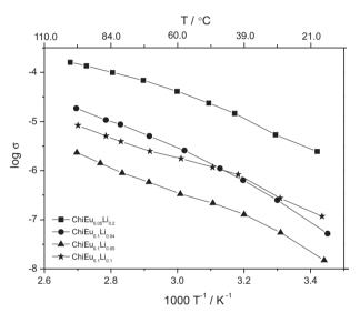
Figure 4. Conductivity plot of the ChiEu<sub>n</sub>Li<sub>m</sub> samples.
