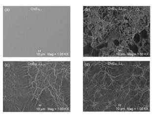
Figure 3. SEM micrographs of the  $ChiEu_{0.1}(a)$  and  $ChiEu_{0.1}Li_m$  for m = 0.04 (b); 0.05 (c) and 0.1 (d) samples.
