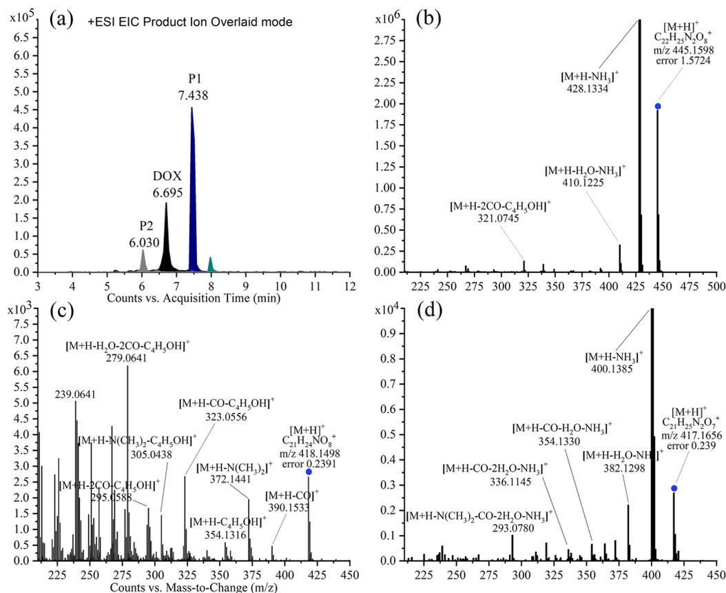
**Figure 5.** Characterization of degraded products from doxycycline in saline medium for *E. cloacae* after 96 h. (a) Extracted ion chromatogram, (b) doxycycline mass spectra ( $t_R = 7.438$  min), (c) product P1 mass spectrum ( $t_R = 6.030$  min) and (d) product P2 mass spectrum ( $t_R = 6.030$  min).
