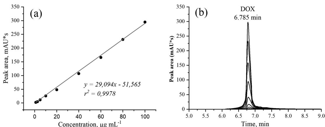
**Figure 3.** Linearity of the method in the quantitative analysis of doxycycline by HPLC-UV. (a) Calibration curve obtained from standard doxycycline solutions, (b) chromatograms overlay obtained from standard solutions at different concentrations.
