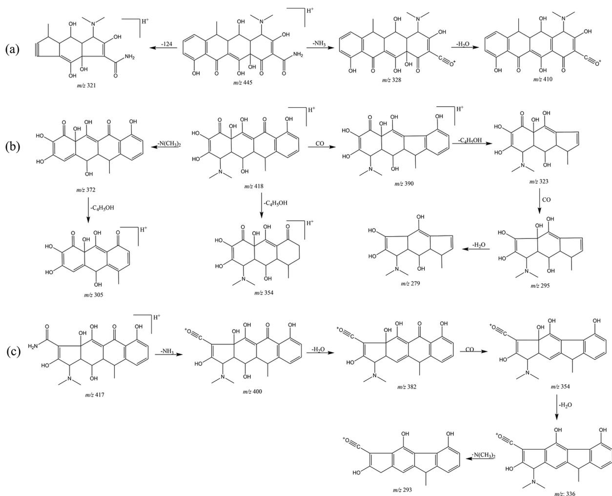
**Figure 6.** Proposed mass fragmentation pattern. (a) Doxycycline, (b) product P1, and (c) product P2.
