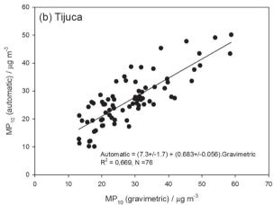
**Figure 2.** Comparison between  $PM_{10}$  mass results from our gravimetric results and the beta attenuation results obtained for (a) Duque de Caxias and (b) Tijuca.
