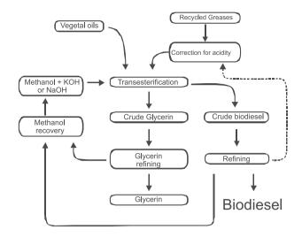
Figure 12. Schematic process for biodiesel production.
