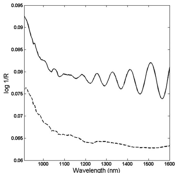
Figure 7. Packaging spectra. (—) PVC film; (---) vacuum packaging.
