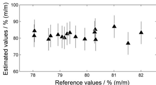
**Figure 5.** Confidence intervals for some validation samples, with 95% of confidence, obtained for the PLSR model developed with the reflectance data.
