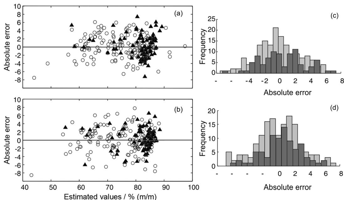
**Figure 3.** Distributions of the absolute errors obtained with the PLSR model developed with the absorbance (a) and reflectance data (b) against the estimated cocaine content values. Calibration (O) and validation samples (▲). Histograms of the absolute errors obtained with the absorbance (c) and reflectance (d) PLSR models (calibration data (light grey bars) and validation data (dark grey bars)).
