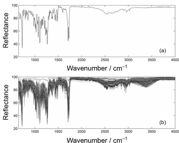
**Figure 1.** ATR-FTIR spectra of (a) cocaine hydrochloride standard and (b) the 184 drug samples used for model development.
