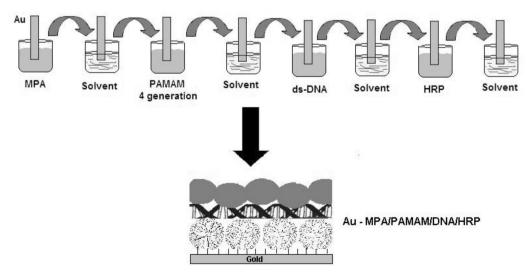
Figure 1. Schematic representation of the process of the film preparation and the materials involved.
